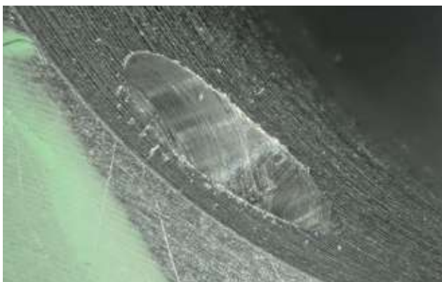
Bore exit after using a standard drill in aluminum
