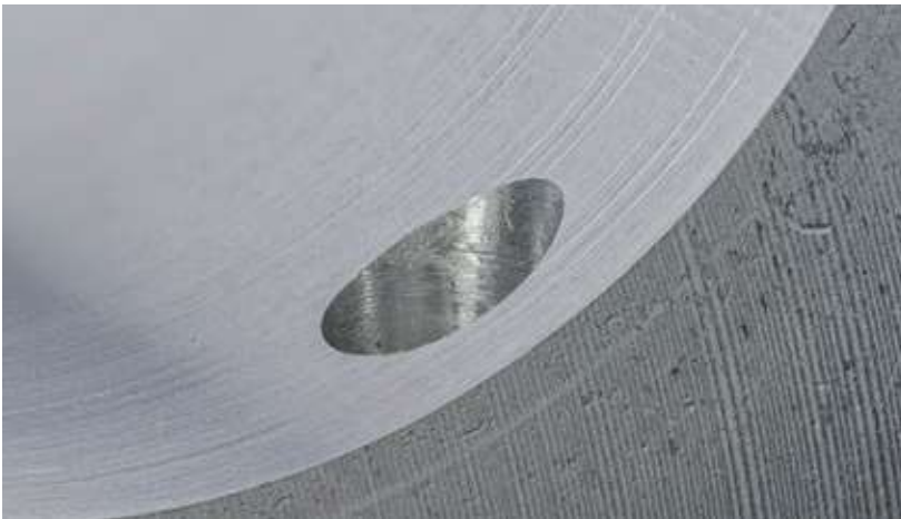
ABOVE: Off-axis bore exit into the cross bore in an aluminum component. With the Ex-BurrDrill, almost no burr can be measured even with this type of machining.
